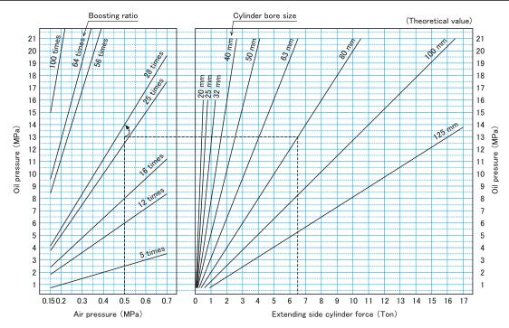
Determine the boosting ratio of Rush Booster and discharge oil amount from each of the operating air pressure, required force, and hydraulic cylinder diameter.
