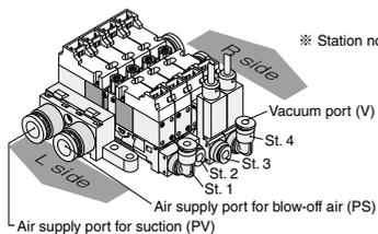
※ Station no. is arranged St.1, St.2 ... St.10 from L side.
