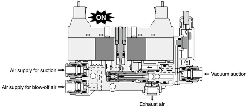
③ Blow-off valve: ON (At blow-off air supply)
