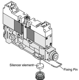
■ Use a Phillips screwdriver to remove a blow-off valve in order to replace silencer elements (Model code: VN013B19) of manifold type. Insert the pin properly after the replacement, make sure the seal rubbers of the valve in the proper position and tighten the fixing screws firmly with the tightening torque 0.15-0.2Nm.
