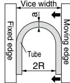
Fix the tube as the left figure shows. Slowly move the moving edge toward the fixed edge. When "a" deforms 25% from the initial value, the measured R is Minimum Installation Radius.
