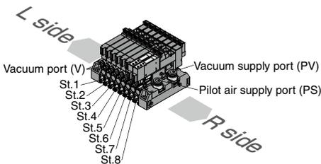
※ Station no. is arranged St.1, St.2 ... St.10 from L side.
