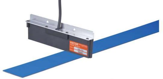
Magnetic Tape Guidance AGV's route can be constructed in various locations, since the magnetic tape route can be constructed where the floor can not be carved. Modification of a magnetic tape route can be done easily and the route is durable against dust, water and light. Guide sensor detects the slight magnetic flux from a magnetic guide tape at operation distance 30mm(20mm to 40mm) and generates multiple switching signals or deviation voltage.
