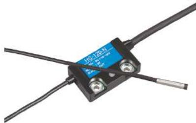
H series sensors are suitable for a reference point sensor of a precision machine. Adopting a N-pole and S-pole borderline magnet as a reference point target magnet, H series sensor generates analog signal or switching signal. The repeatability at the borderline of N-pole and S-pole of target magnet is  $\pm 0.1\mu\text{m}$ .
