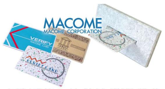
6mm dot N-pole and S-pole data are magnetized on a Barium-Ferrite card. Polarity distinguishable switches are built-in EK series corresponding to each dot on the card. Each switch generates signal ON for N-pole dot and OFF for S-pole dot. The non-contact reading method realizes high durability to harsh environments. The magnetized data on the Barium-Ferrite card are more durable than a normal magnetic stripe card.
