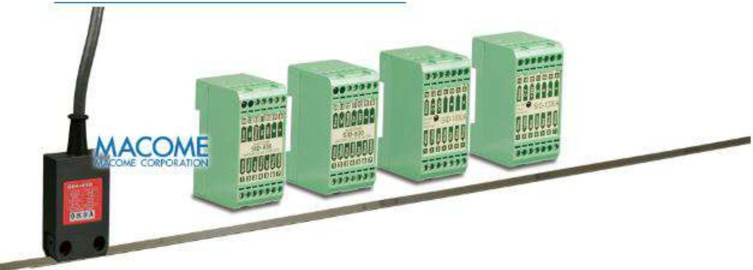
MACOME Scale is consisted of Scale, Head and Detector. Magnetic graduations magnetized on the Scale at an interval of 4mm pitch are read out by Head at Operation distance 0.3mm (0.05mm to 0.55mm) as AB phase sinusoidal voltage. The signal are interpolated 1/10, 1/20 or 1/100 by Detector to generate AB phase signal.
