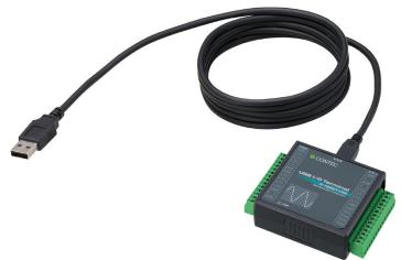
This product is a USB2.0 compatible terminal module that extends the analog I/O function of USB port of PCs. 8ch/16bits analog inputs are employed and signal lines can be directly connected to the screw terminals in the system. Compact design to match Note PCs and excellent in mobility as operation is powered by USB bus. This product accompanies Windows driver and full-fledged data logger software "C-LOGGER".
