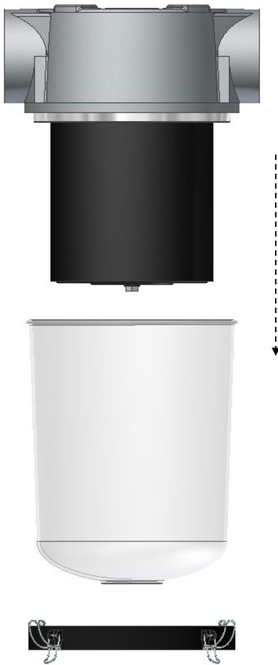
Figure C.2.3: ST bucket removal.
