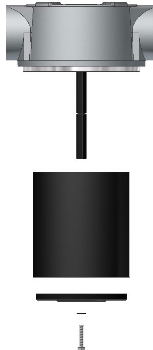
Figure C.3.2: Element and top plate removal.
