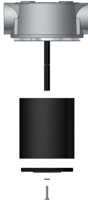
Figure C.3.2: Element and top plate removal.
