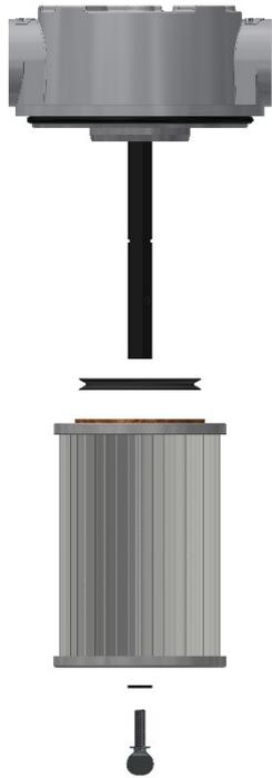
Figure C.3.1: Element removal.
