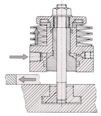
It will be in a unclamp state by contracting a conical claw by supply of oil pressure from a port.
