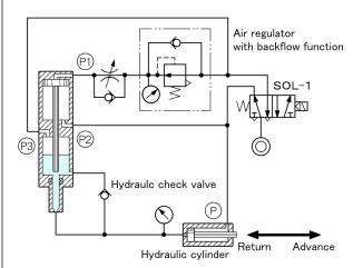
This circuit is a circuit when high thrust ia required only at the start such as removing the biting part at the start of advance movement and then moving in fast advance.  $\circ$
