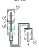
When the  $\widehat{\mathbb{P}3}$  port is supplied with compressed air, the hydraulic cylinder is fast–forwarded by the oil in the oil tank.
